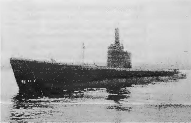
The Gato-class submarine was the state of the art in American design at the start of World War II. Using the previous Tambor-class submarine as a basis, Gatos incorporated improvements to increase their overall patrol and combat abilities. Modifications to the diesel engines and batteries increased patrol duration over Tambors, and internal alterations provided more amenities for the crew. The class is named after its lead ship, USS Gato (SS-212).
