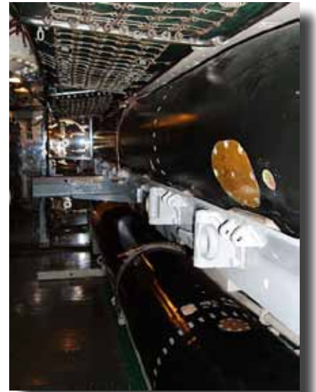
Two Mark 14 torpedoes stored in the after torpedo room of the museum ship USS Pampanito
