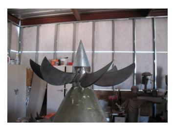
A seven-bladed, scmitar shaped propeller as declssified on models of the Sturgeon-class boats is shown attached to the aft hull. The propeller and "duce cap" will be bronze colored.
