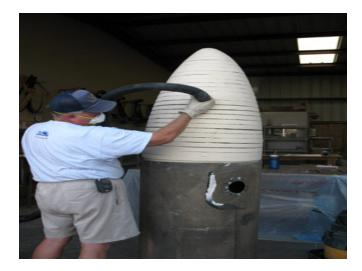
Shipmate Howard Doyle sands the stacked foam sheets that form the bow section of the model. Fiberglass will be molded over the foam sections for a smooth hull finish. The sail and planes will be constructed similarly.
